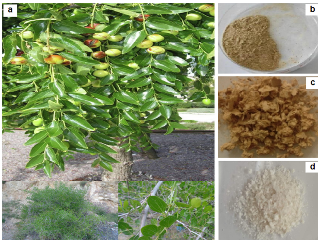
Figure 1. Photographs of (a) Ziziphus jujuba plant, (b) untreated Ziziphus jujuba material, (c) alkali-treated samples and (d) final bleached cellulose.
